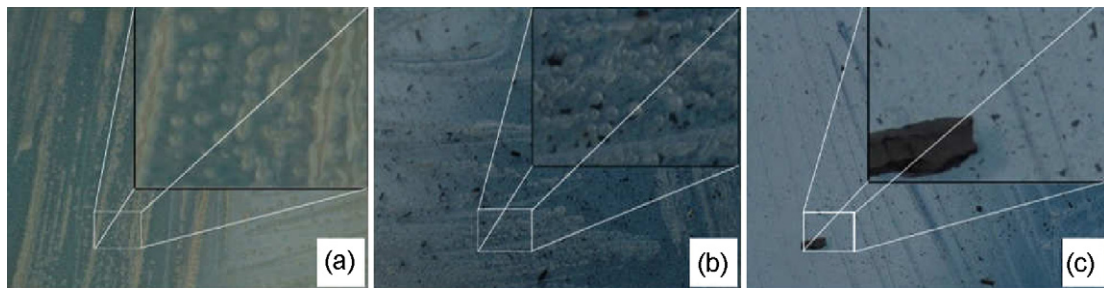
Fig. 8. Test samples for strains of E. coli in the agar dish for negative control (a), presence of AC (b) and presence of AgAC (c). The white colonies on figure (a) and (b) (see the insets for more detailed) show that the negative control allowed normal growth and AC did not inhibit the growth. No colony is observed in figure (c) confirming a strong inhibition against the growth of AgAC on E. coli .
